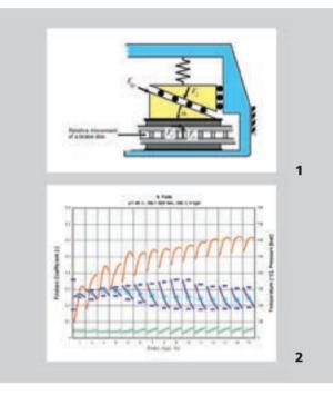
Operating principle of a selfenergizing disc brake with a constant wedge angle.
