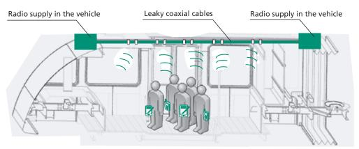
Leaky coaxial cables installed in the AutoTram<sup>®</sup> for radio propagation and positioning.
