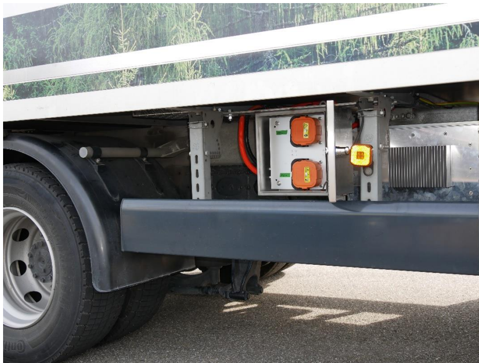
The DC chopper sits under the truck box to save space. © Fraunhofer ISE
