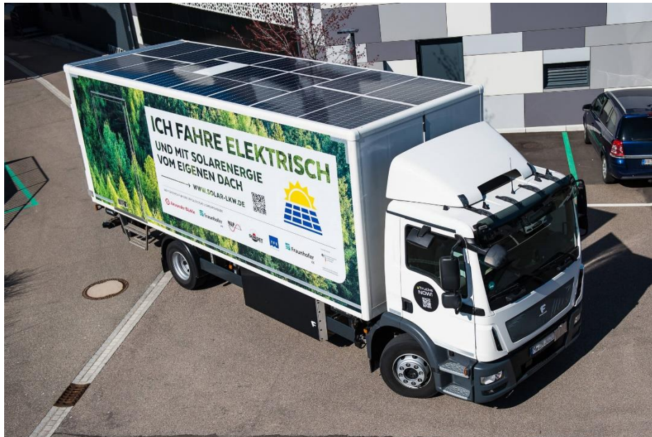
The solar modules integrated into the box body make full use of the entire roof © Fraunhofer ISE
